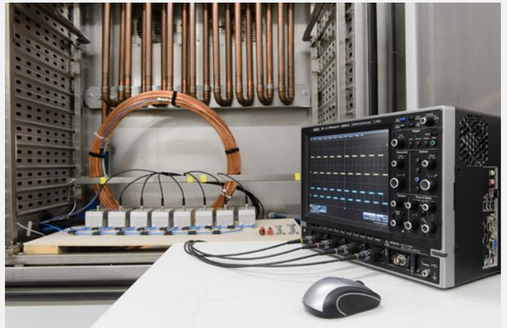
Fig. 4: Calibration of multiple gas quality sensors [6]
